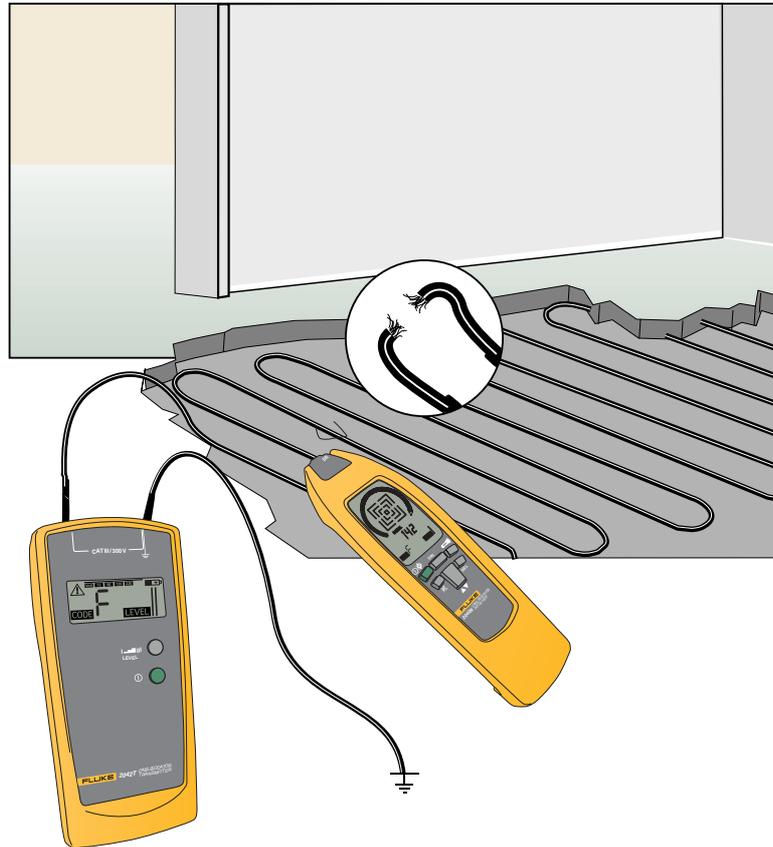
Locating faults in electrical under-floor heating
