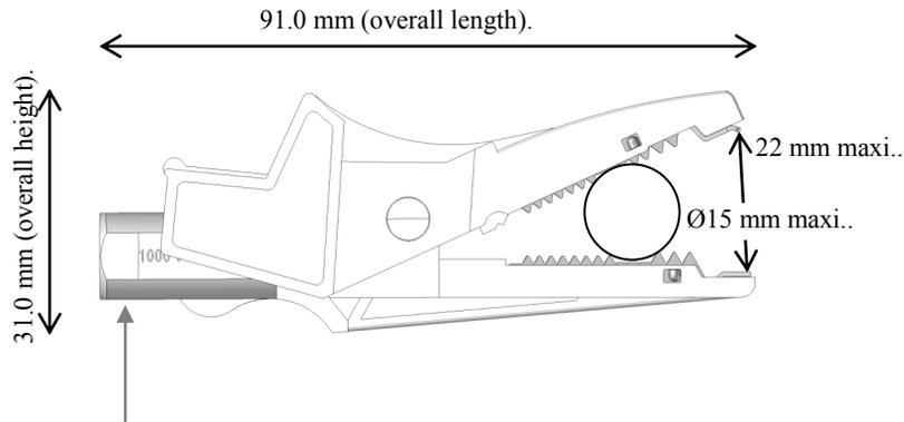
The 4 mm banana female connection complies with the 4 mm banana plugs of most of the worldwide most famous manufacturers.
